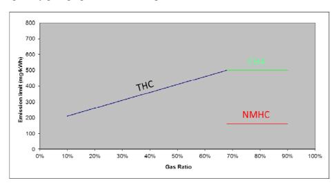
figure 1: illustration of the HC limits in the case of a HDDF type2 engine operating in dual-fuel mode during the WHTC cycle (natural gas dual-fuel engines)
