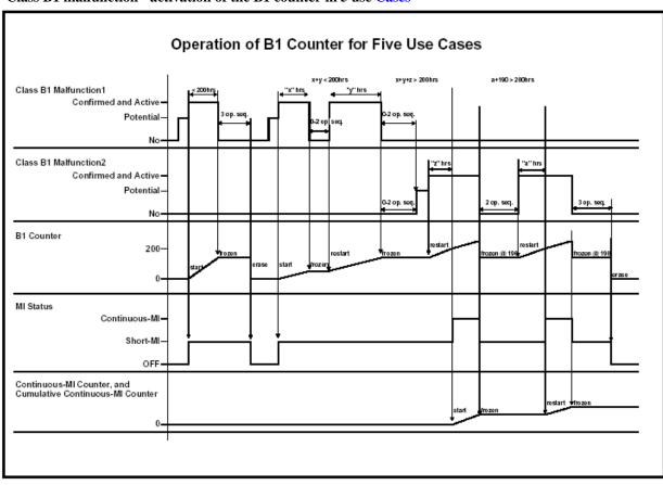
Figure 5 Class B1 malfunction - activation of the B1 counter in 5 use Cases
