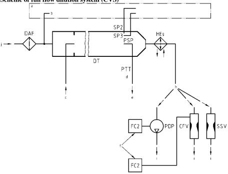
a = analyzer system b = background air c = exhaust d = details see Figure 17 e = to double dilution system f = if EFC is used i = vent g = optional h = or
