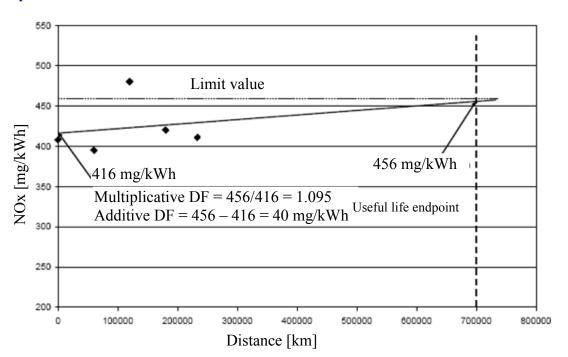
Figure 1 Example of deterioration factor determination
