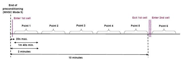
Figures 5 and 6 WNTE test cycle grids
