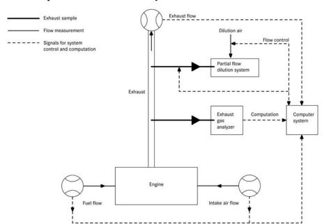
Figure 6: Scheme of raw/partial flow measurement system
