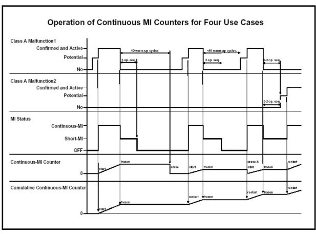
Figure 4A Class A malfunction - activation of the MI and MI counters
