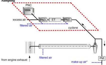
\* Alternatively, the control software might account for the flow removed by the PN system
