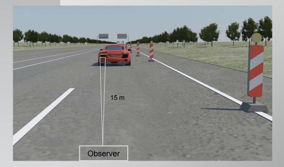
The observer needs a distance of more than 125 meters to see the row of line poles under the same visual angle.
