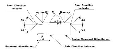
(\*\*) The value of 5° given for the dead angle of visibility to the rear of the side direction-indicator is an upper limit.  $d \le 2.50$  m
