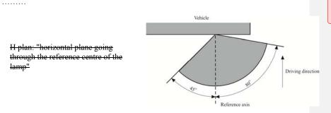
Categories 2a and 2b:Direction indicators for the rear of the vehicleCategory 2a:Rear direction indicator lamps with steady luminous intensityCategory 2b:Rear direction indicator lamps with variable luminous intensity
