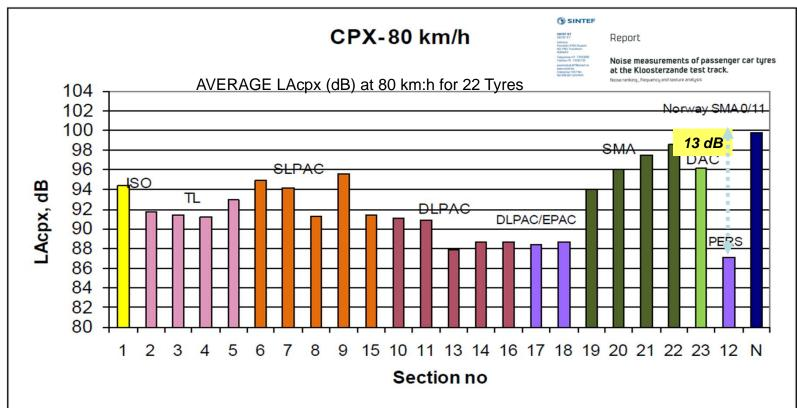
Between the noisiest tyre on the noisiest road surface (Tyre 16 on SMA 0/16) and the quietest tyre on the quietest road surface (Tyre 12 on Rollpave PERS), there is a noise difference of approximately 17 dB at both 50 and 80 km/h. Even between tyre 16 on the SMA 0/16 and tyre 12 on a more commonly used surface as the double layer PAC (section 16), there is a difference of 14-15 dB.
