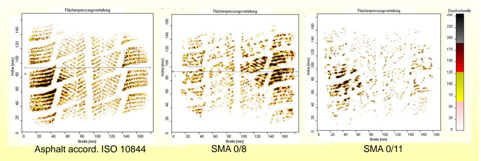
Pressure in the foot print on different road surfaces
