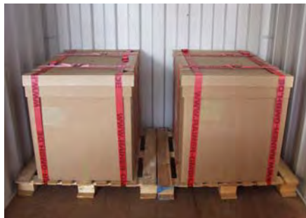
Figure 10-7 : Cargo firmly secured to pallets by textile lashings
