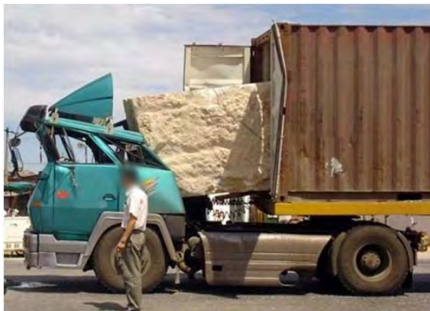
Figure 4-1 : Lack of longitudinal securing
