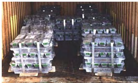
Figure 10-16 : Metal ingots compacted by steel banding (securing not completed)
