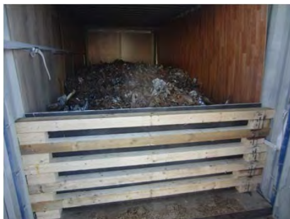
Figure 10-44 : Lined container loaded with scrap
