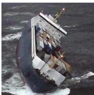
Figure 4-5 : heavily listing vessel after a partial cargo shifting
