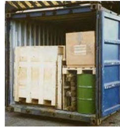
Figure 10-25 : Mixed stow, use of pallets
