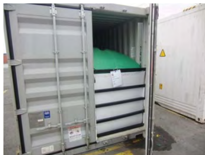
Figure 10-40 : Container fitted with flexitank
