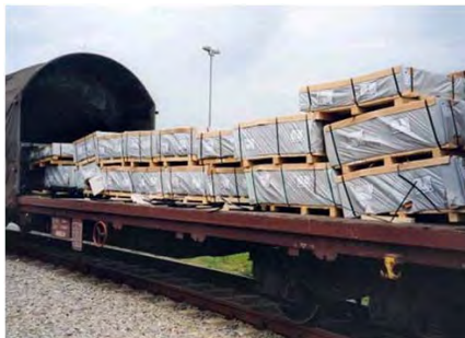
Figure 4-7 : Loose packages on rail wagon
