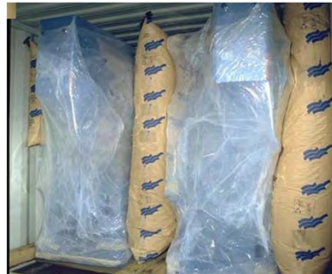
Figure 10-9 : Irregular shaped packages blocked with dunnage bags
