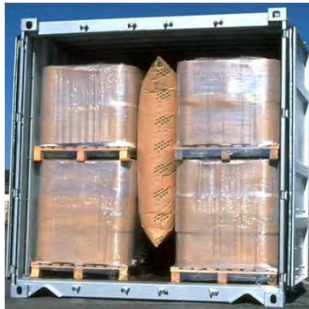
Figure 10-8 :Gap filled with a central dunnage bag
