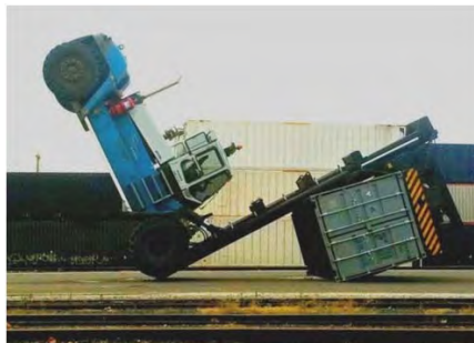
Figure 4-14 : Tipped container handler (© abc.net.au)
