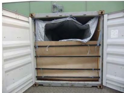
Figure 10-43 : Container with bulk material liner
