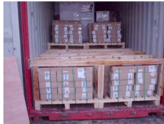
Figure 10-1 : temporary floor in a container
