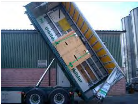
The cargo securing arrangement of a heat exchanger is here tested for acceleration forces forward and sideways.
