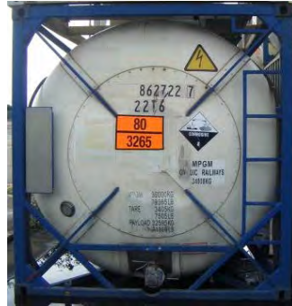
Figure X-2 : Partial frame ladder
