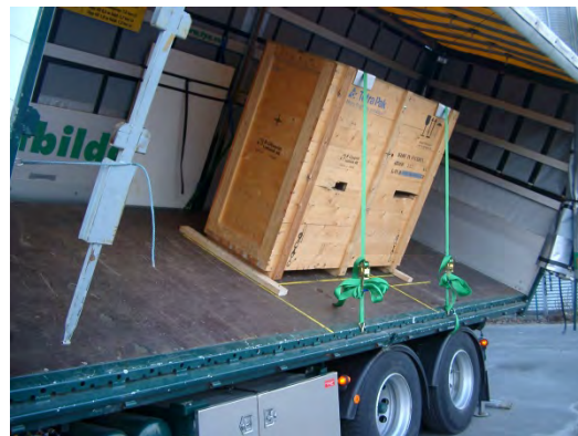
The cargo securing arrangement of a heat exchanger is here tested for acceleration forces forward and sideways.
