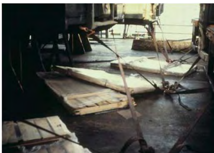
Figure 4-3 : Cargo having broken out of a trailer Loose cargo on Ro-Ro vessel
