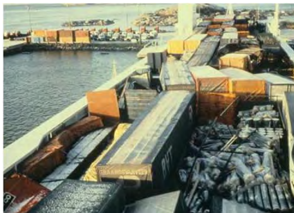
Figure 4-4 : Spilled/Shifted cargo on a Ro-Ro deck
