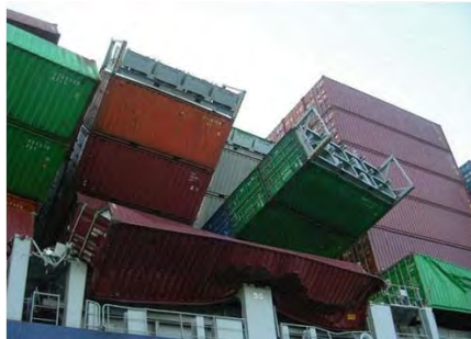
Figure 4-15 : Failed stack of containers (© KIMO International)
