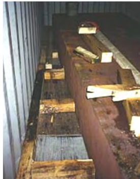
Figure 10-34 : Transverse blocking of steel slab
