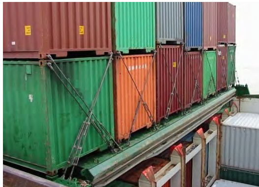
Figure 13-2 : Cell guides and lashing rods
