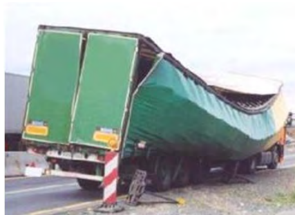
Figure 4-2 : Inadequate side wall strength
