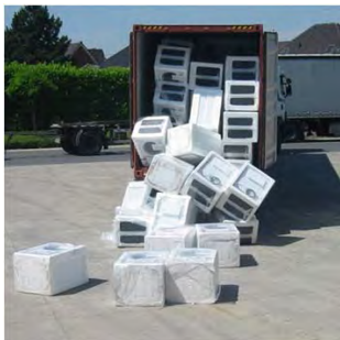
Figure 4-6 : Unsecured packages, falling out when the doors are opened
