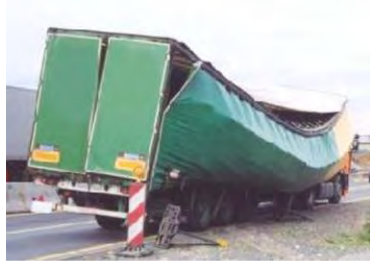
Figure 4-2 : Inadequate side wall strength
