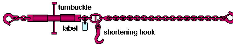
Figure 10-15 : Standard chain lashing with shortening hook
