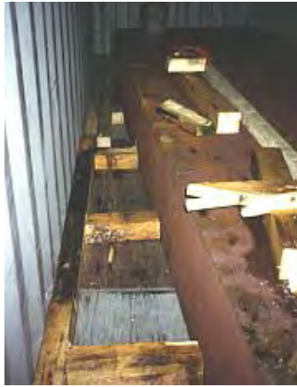
Figure 10-34 : Transverse blocking of steel slab
