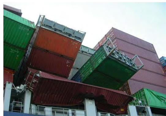
Figure 4-15 : Failed stack of containers (© KIMO International)
