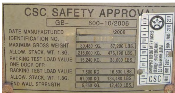
Figure 9-3 : CSC safety approval plate with next examination date
