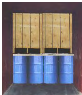
Figure 10-24 : Mixed stow, dry over wet goods
