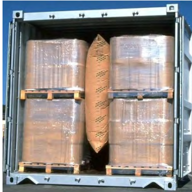
Figure 10-8 :Gap filled with a central dunnage bag
