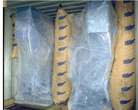
Figure 10-9 : Irregular shaped packages blocked with dunnage bags
