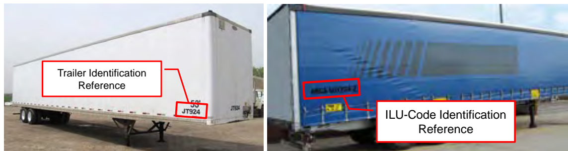
Figure 14-1 : Three examples of CTU identification references
