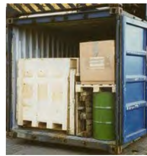
Figure 10-25 : Mixed stow, use of pallets
