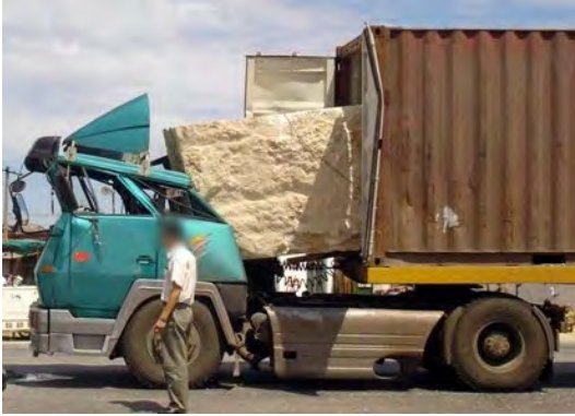
Figure 4-1 : Lack of longitudinal securing
