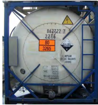
Figure X-2 : Partial frame ladder
