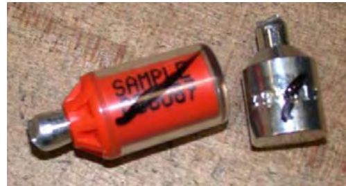
Figure XI-29 : Cut bolt seals - head
