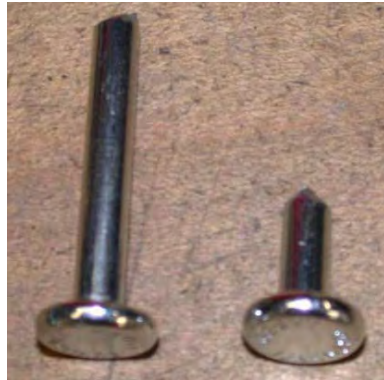
Figure XI-28 : Cut bolt seal - stems
