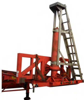
Figure X-9 : Trailer mounted access ladder
