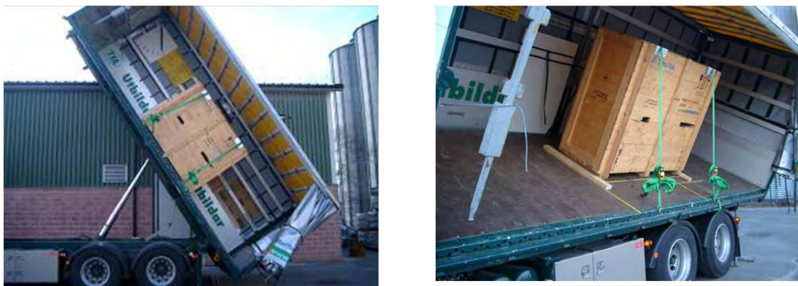
The cargo securing arrangement of a heat exchanger is here tested for acceleration forces forward and sideways.
