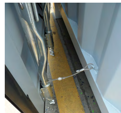
Figure XII-22 : Door retaining strap
