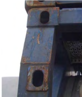
Figure XV.58 Swap tank corner post stepped back fitting
