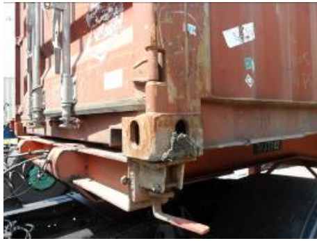
Figure XIX.2 : Mud in corner fitting
