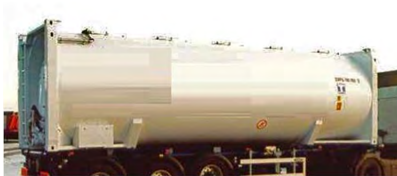
Figure XV.60 Pressurised powder swap tank
