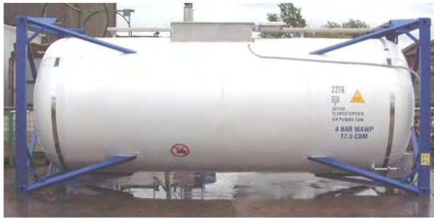
Figure XV.48 Beam tank no top rail
