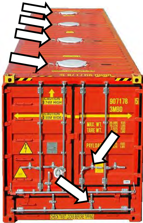
Figure XI-10 : Dry bulk sealing points
