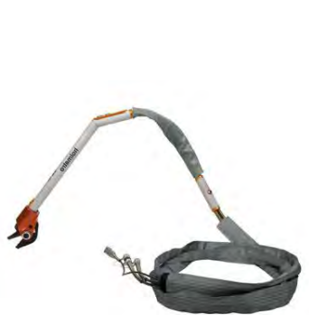
Figure XI-35 : Hydraulic cutting head
