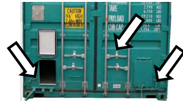
Figure XI-12 : Dry bulk discharge hatch (rear)
