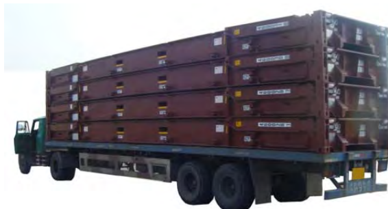
Figure XV.40 Stack of 40ft folding end flatracks
