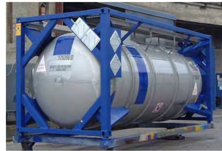
Figure XV.49 Beam tank with top rail
