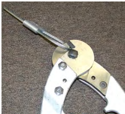
Figure XI-25 : Cutters for cable seal
