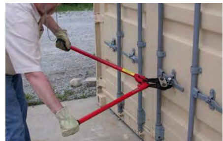
Figure XII-3 : Cutting a seal on the ground
