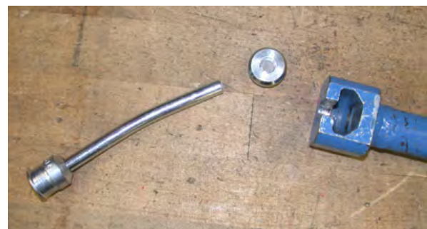
Figure XI-33 ; Rail car bolt seal and breaking tool
