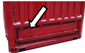
Figure XI-13 : Dry bulk discharge hatch (front)
