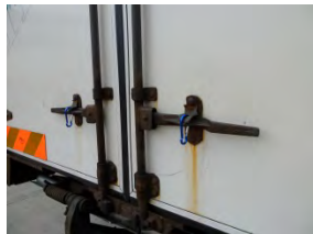
Figure XI-5 : Surface mounted handles
