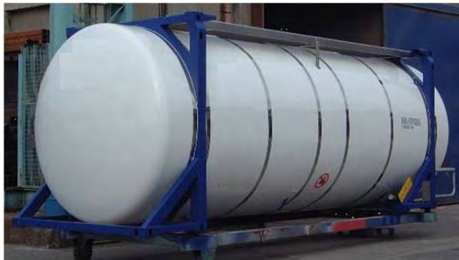
Figure XV.59 Swap tank showing exposed ends
