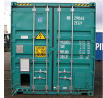
Figure XV.23 Cat flap type hatch in rear doors
