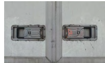
Figure XI-7 : Recessed handled with protruding eyes
