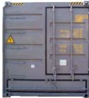
Figure XV.22 letterbox type hatch in fixed rear end
