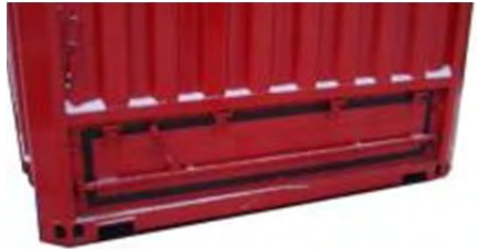
Figure XV.21 Letterbox type hatch in container front wall
