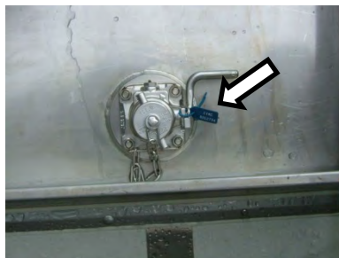
Figure XI-16 : Top valve seal
