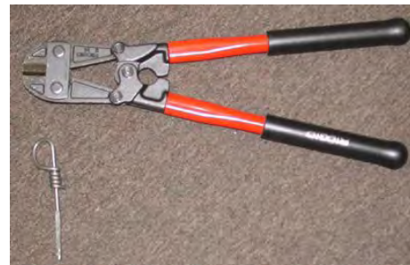
Figure XI-26 : Cutters for twist seal
