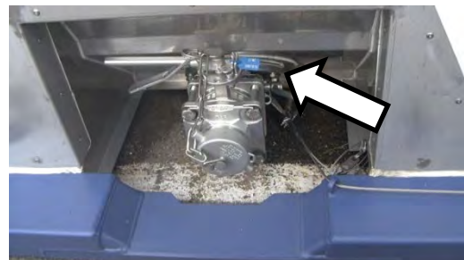
Figure XI-17 : Discharge valve seal
