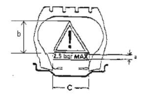
$\begin{array}{l} a=2 \text{ mm min (height of lettering)} \\ b=12 \text{ mm min for tyre section height} \leq 120 \text{ mm} \\ 18 \text{ mm min for tyre section height} > 120 \text{ mm} \\ c=14 \text{ mm min (width of lettering)} \end{array}$
