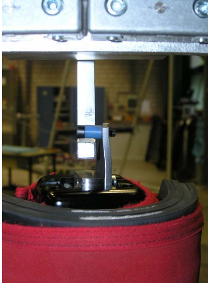
Fig. 9: Modified support bracket for impact angle variation of +10^\circ (view in impact direction)
