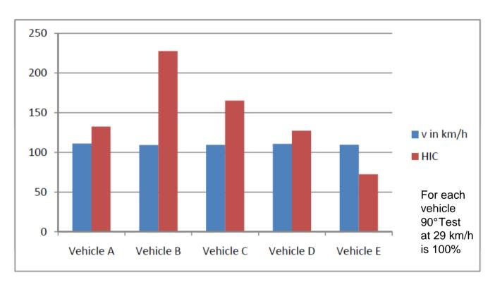
Test results of vehicles designed for 32km/h oblique condition compared to the same car designed for 29 km/h 90°. Perpendicular is always 100%.
