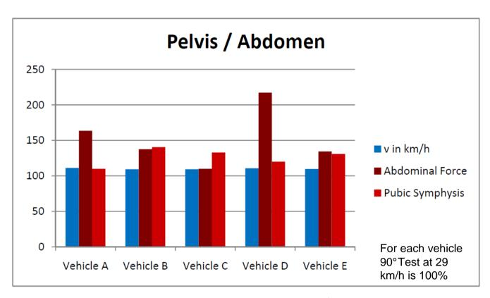
Test results of vehicles designed for 32km/h oblique condition compared to the same car designed for 29 km/h 90°. Perpendicular is always 100%.
