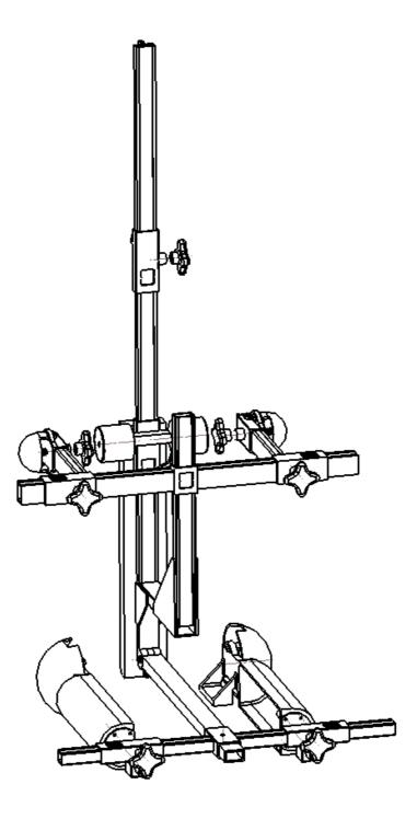
Figure 3 : 3D view of the measuring device.
