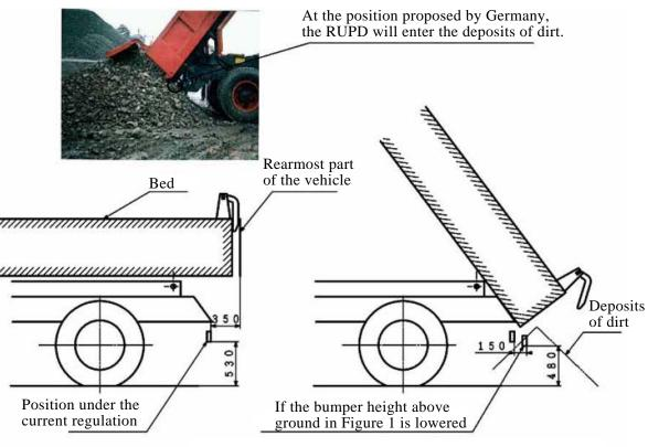
Figure 2 RUPD Entering the Deposits of Dirt at Dumping
