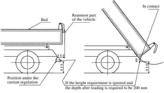
Figure 1 Contact Caused by Dumping
