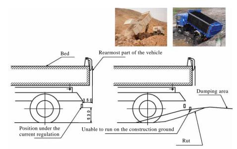
Figure 4 Unable to Run on Unpaved Roads in Construction Sites, Dump Yards, etc.
