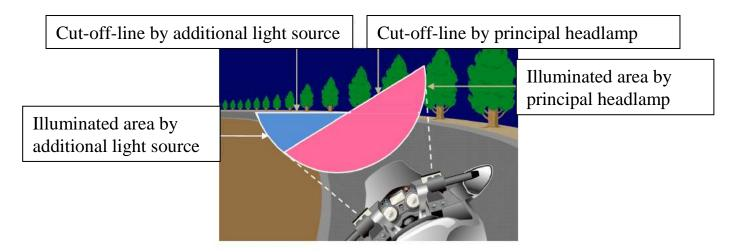
Fig.2 Additional light source type headlamp
