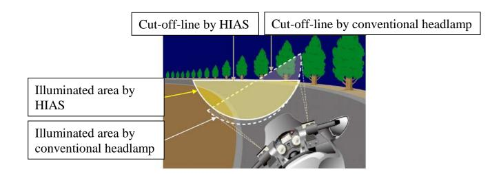
Fig.1 Horizontal inclination adjustment system (HIAS)
