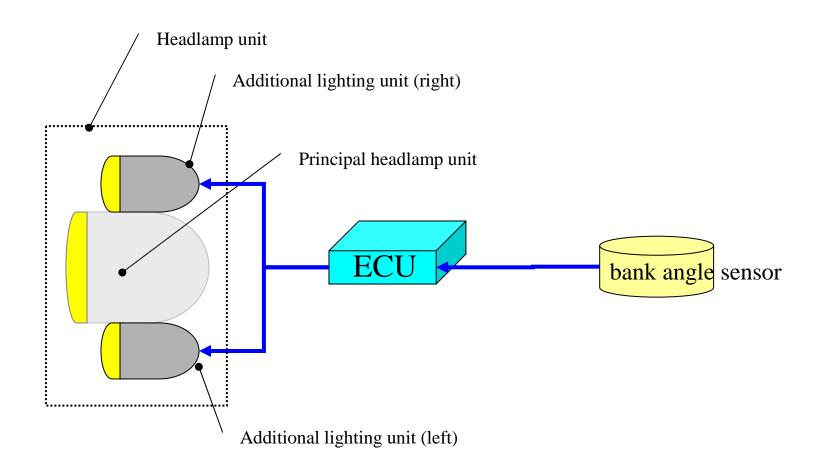
Fig.3 System block diagram (example)
