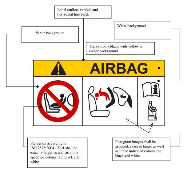
The overall dimensions shall be at least 120 x 60 mm or the equivalent area.
