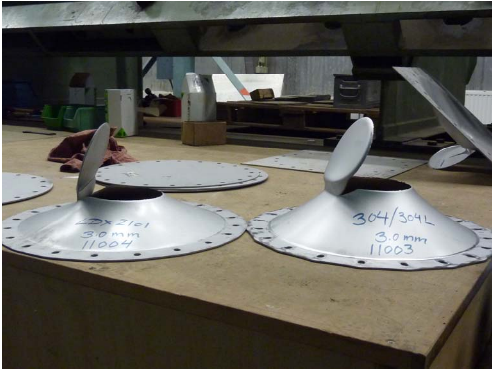
Figure 6 Test specimens after fracture, showing an austenitic stainless grade to the right and an austenitic-ferritic grade to the left. The diameter of the specimens is about Ø500 mm.
