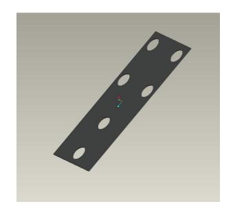
Current segment fit is fine tuned with 0.05 mm thick shims Will have 0.1 and 0.2 mm thick shims to reduce number of shims and help handling
