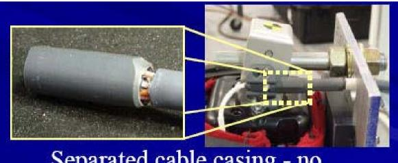
Separated cable casing - no data loss
