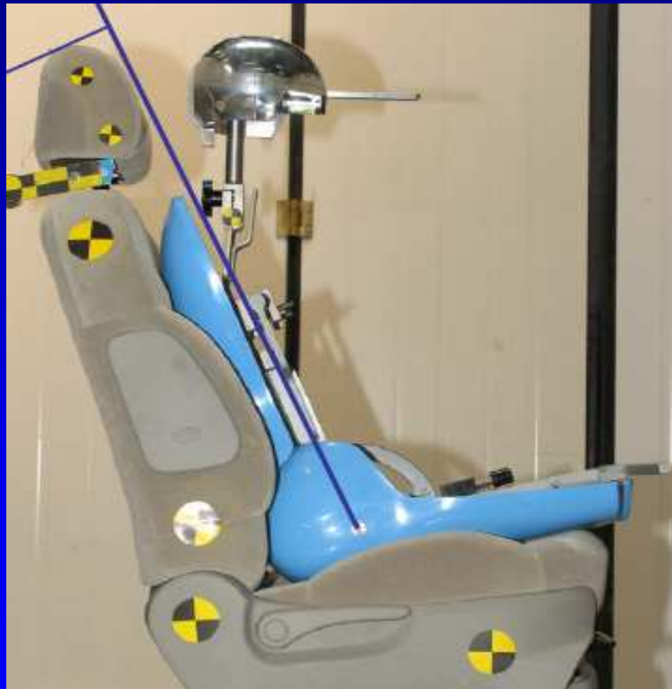
Fig.1: UN-ECE Regulation 17 method for measuring head restraint height
