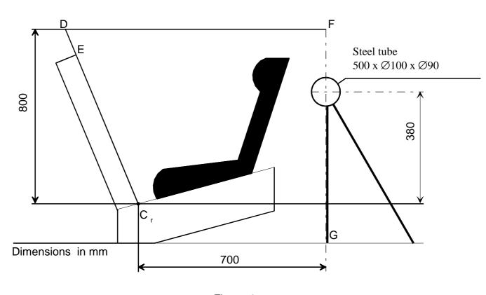
Figure 4: Arrangement for testing rearward-facing devices, except group 0, not supported by the dashboard
