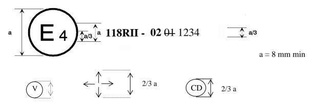
The above approval mark affixed to a component shows that the type concerned was approved in the Netherlands (E4) pursuant to Part II of Regulation No. 118 under approval number 01 021234. The first two digits (01 02) of the approval number indicate that the approval was granted in accordance with the requirements of the 01 02 series of amendments to Regulation No. 118.
