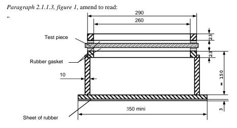
Figure 1: Support for ball tests"
