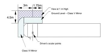
Figure 8e: Class VI mirror partially covering additional field of vision at 1 m high"
