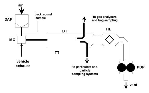
Full Flow Dilution System with Positive Displacement Pump
