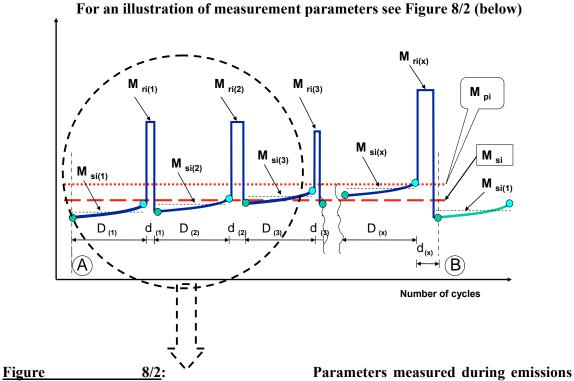
test during and between cycles where regeneration occurs (schematic example)
