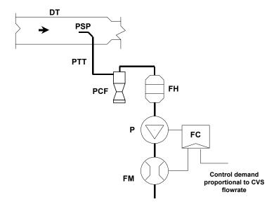
Figure 12: Particulate Sampling System
