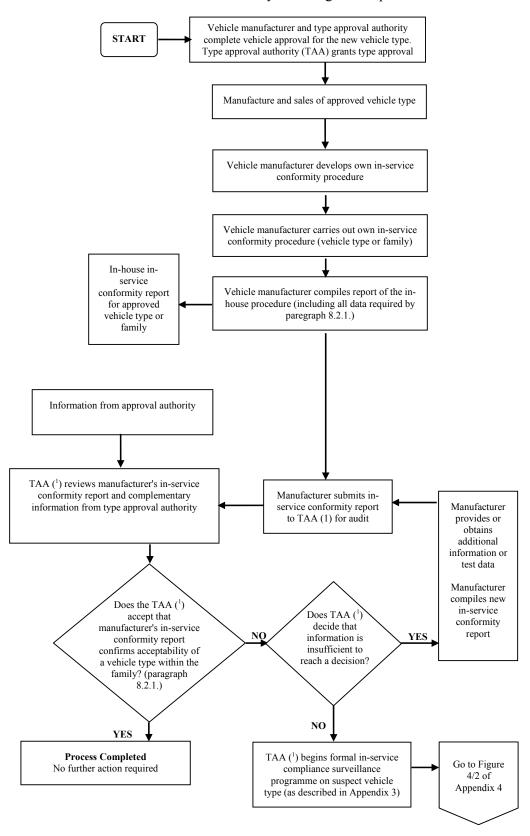
$\underline{\text{Figure 4/2}}$  In-service conformity testing - selection and test of vehicle
