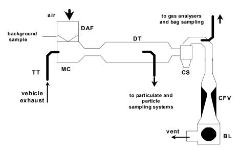
Full Flow Dilution System with Critical Flow Venturi
