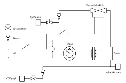
Figure 11: NOx Converter Efficiency Test Configuration
