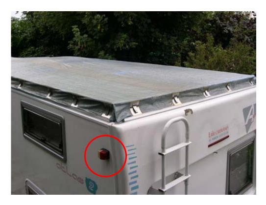
It is clear that in this case the  $45^{\circ}$  angle of visibility to the inside (imposed by ECE R7 approval as position lamp) is useless.
