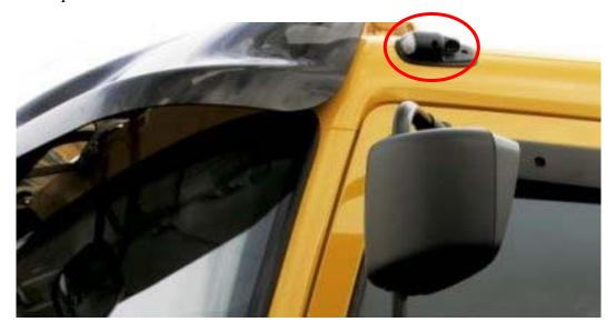
As for the preceding example, it is clear that in this case the  $45^{\circ}$  angle of visibility to the inside (imposed by ECE R7 approval as position lamp) is useless.
