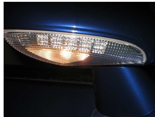
courtesy lamp integrated in outer mirror
