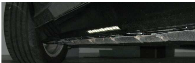
courtesy lamp integrated in side skirt with leds
