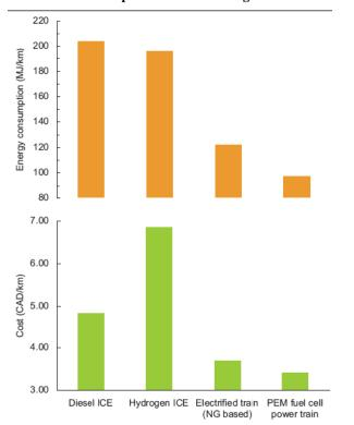
Energy consumption (upper graph) and corresponding travel cost (lower graph) of trains with various power train technologies
