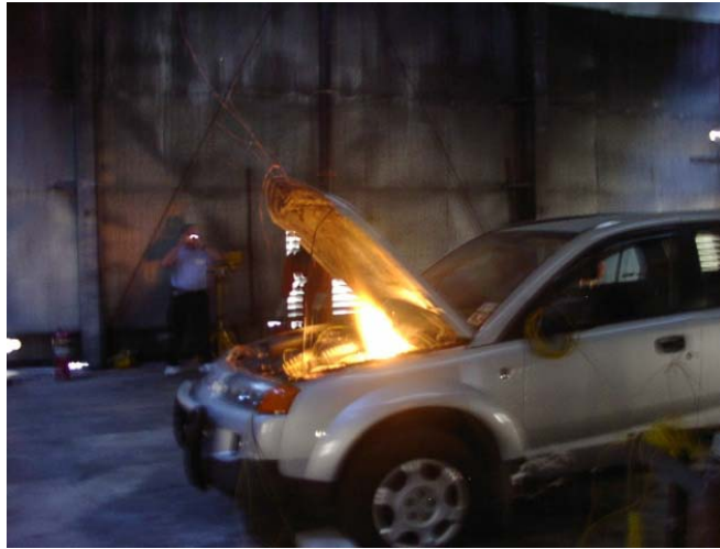
Figure 2: Fuel Line Leakage with Hood Open
