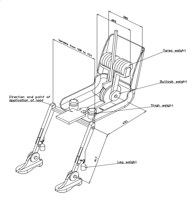
$\underline{Figure~2}$  - Dimensions of the 3-D H machine elements and load distribution (Dimensions in millimeters)
