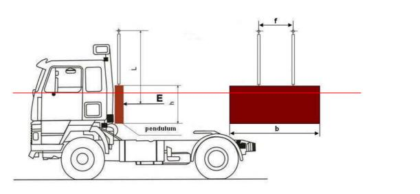
Fig. 4. – Rear-wall strength test
