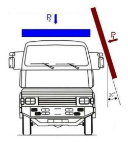
Fig. 3. Roof strength test (Test C).
