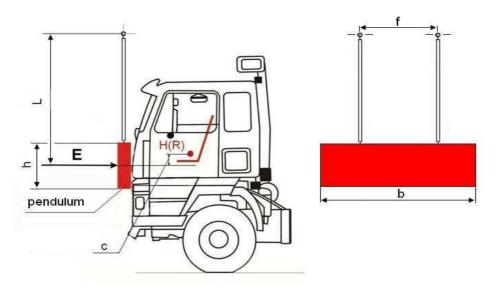
Fig. 1 – Front impact test (test A).
