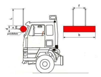
Fig. 2. – Front pillar impact test (Test B).
