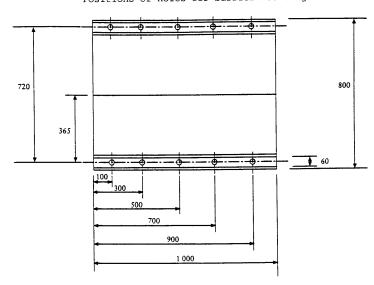
Hole diameters 9.5 mm. All dimensions in mm.
