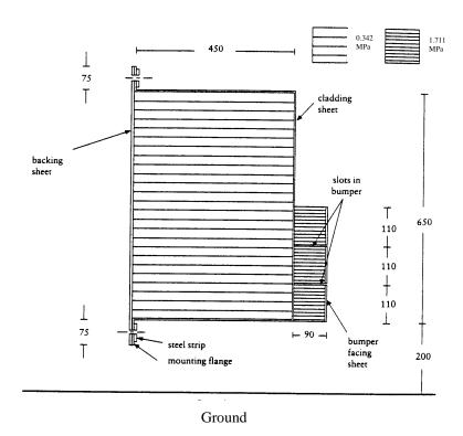
Barrier width: 1 000 mm All dimensions in mm.
