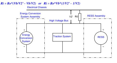
Figure 3: Measurement of V2'
