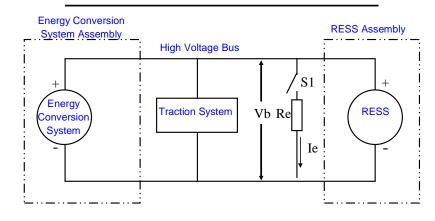
Figure 4: Measurement of high voltage bus energy
