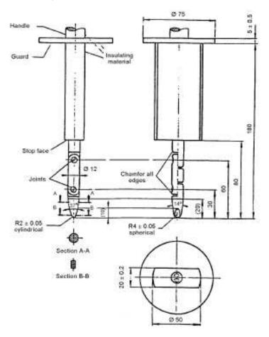
Material: metal, except where otherwise specified Linear dimensions in millimetres
