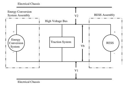
Figure 1: Measurement of Vb, V1, V2
