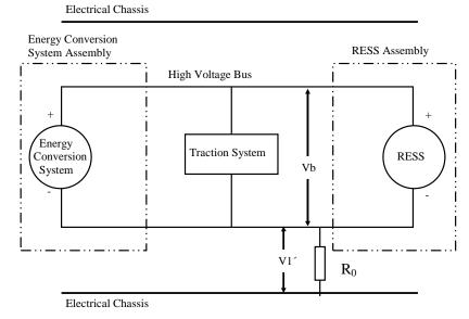
Figure 2: Measurement of V1'
