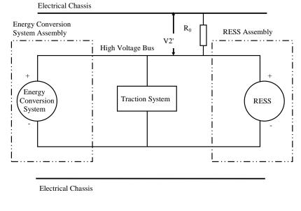
Figure 3: Measurement of V2'
