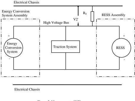
Figure 3: Measurement of V2'
