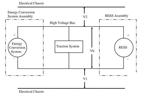
Figure 1: Measurement of Vb, V1, V2
