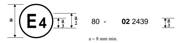
The above approval mark, affixed to a vehicle, shows that this type of vehicle has been approved in the Netherlands (E4) under number 022439 with regard to the strength of the anchorages on the vehicle. The approval number indicates that the approval was granted in accordance with the requirements of Regulation No. 80 as amended by the 02 series of amendments."
