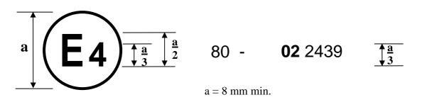
The above approval mark affixed to a seat shows that the seat type concerned has, with regard to the strength of the seats, the test being carried out in accordance with paragraph 2 of annex 4, been approved in the Netherlands (E4) under number 022439. The approval number indicates that the approval was granted in accordance with the requirements of Regulation No. 80 as amended by the 02 series of amendments.
