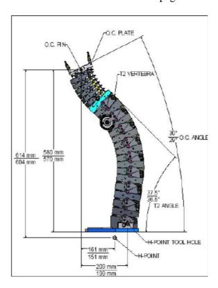
Figure 9-3 Spine curvature check
