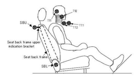
Figure 9-1 Video motion target placements
