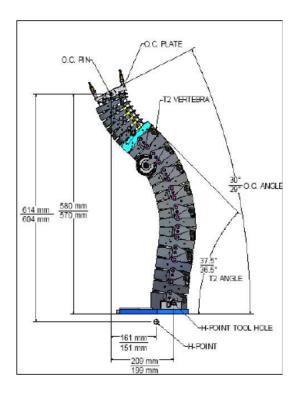
Figure 9-3 Spine curvature check
