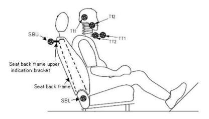
Figure 9-1 Video motion target placements
