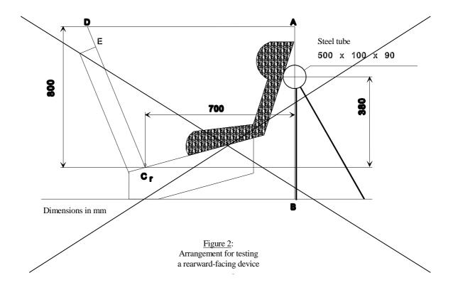
7.1.4.4.1.2.2. <u>Child restraints in group 0 not supported by the dashboard, and carrycots</u>: the head of the manikin shall not pass the planes AB, AD and DE as shown in Figure 3 below. This shall be judged up to 300 ms or the moment that the manikin has come to a definitive standstill whatever occurs first.
