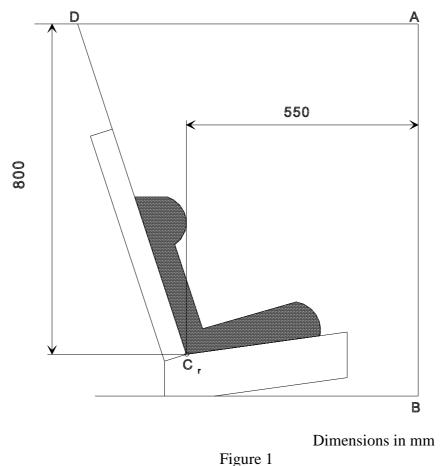
Arrangement for testing a forward-facing device
