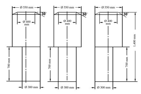
The base of the first cylinder shall be within the projection of the second cylinder. "
