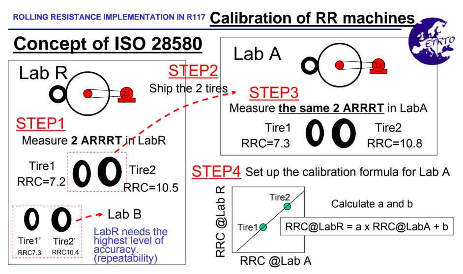
STEP5 LabA can measure any tires for TA purpose. Measured RRC is converted to LabR scale with calibration formula.
