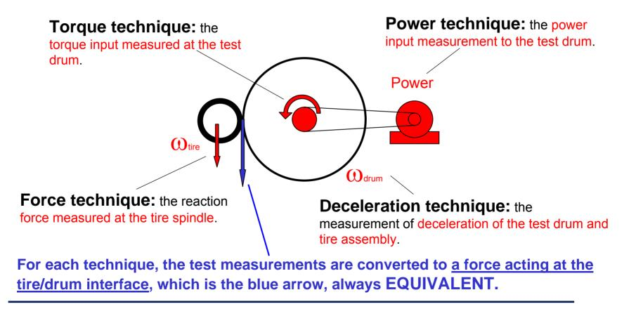
NB : The expression "measuring method" in the standard may be misleading. ISO 28580 describes a single measurement method, with 4 variants for measurement technique for data acquisition.
