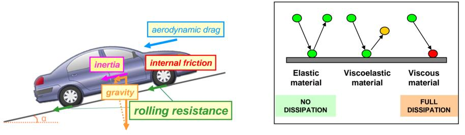
RR is a force acting opposite to the travel direction if a tyre is rolling. Due to the vehicle load, the tyre is deformed in the contact area with the road surface.
