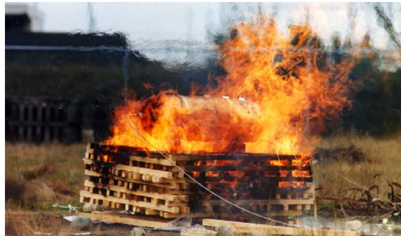
Wood bonfire test of tank
