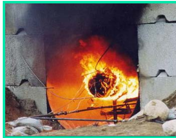
Bonfire test of tank using LPG burner
