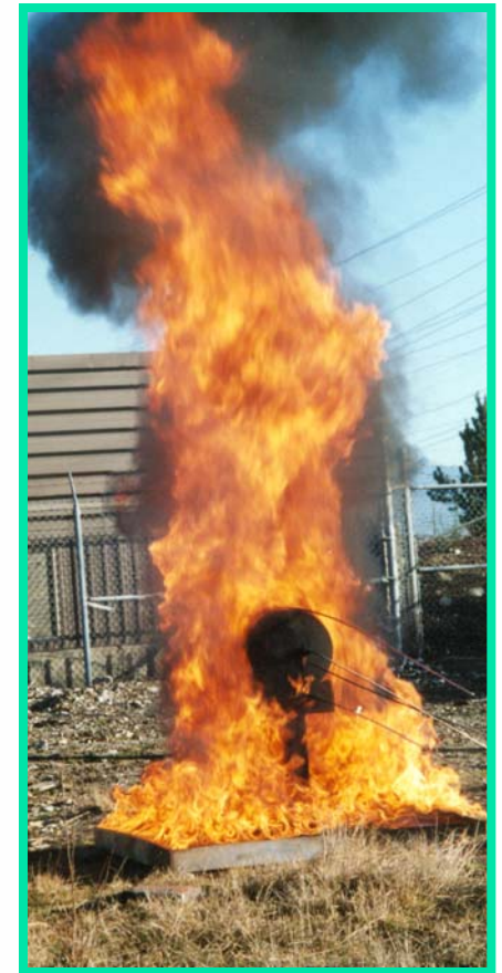
Diesel fuel fire test of tank
