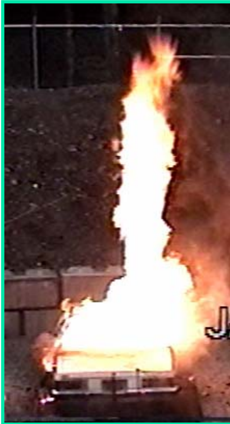
H 2 release from burning vehicle
