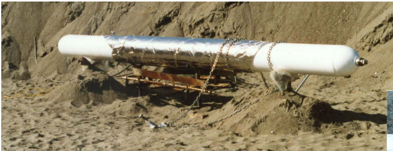
Set-up for bonfire test using LPG burner
