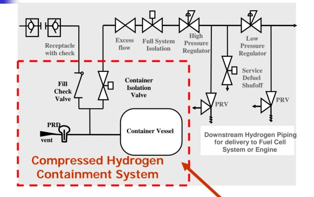
Includes all components and parts that form the primary pressure boundary for stored hydrogen Isolates stored hydrogen from --
