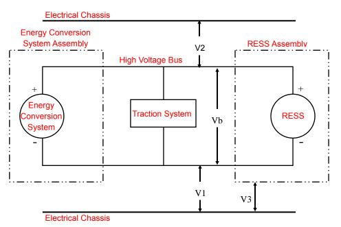
Figure 12: Measurement of Vb, V1, V2
