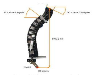
Figure 9-3 Spine curvature check
