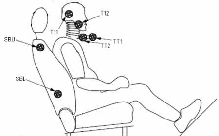
Figure 9-1 Video motion target placements
