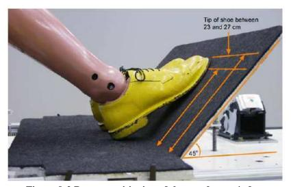
Figure 9-2 Proper positioning of the test dummy's feet.
