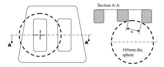
Figure 3-2 - Measurement of a vertical gap "a".
