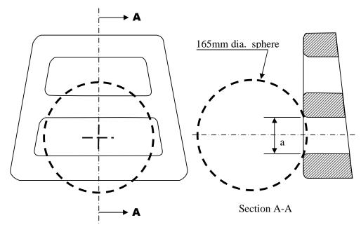
Figure 3-1 - Measurement of a horizontal gap "a".
