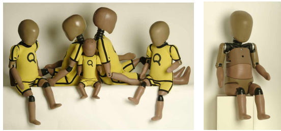
Figure 2. The Q-dummy family: (from left to right) Q1.5, Q3, Q0, Q6, Q1 and Q1 without suit.
