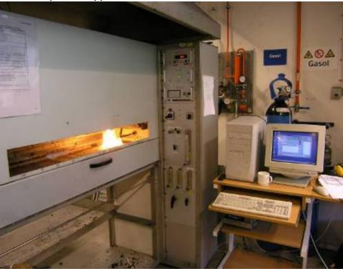
Criterion: Critical Heat Flux at extinguishment  $\geq$  6 kW/m<sup>2</sup>. Same as for floors and external roofs on trains.
