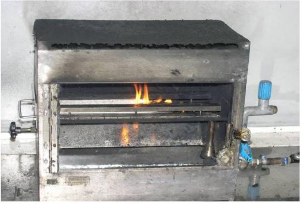
The test only considers horizontal flame propagation, and contains additional technical shortcomings such as interrupted combustion when test object burns too fast and falls apart.
