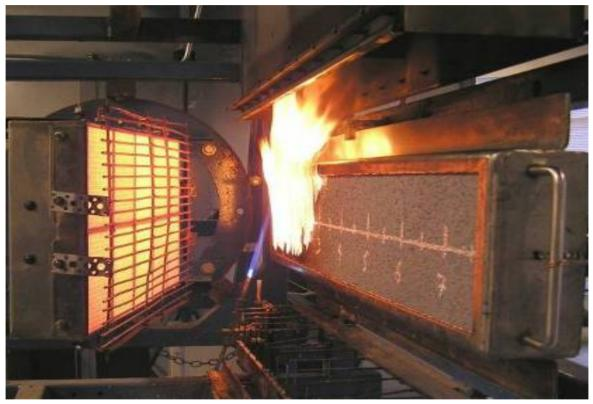
Criterion: Critical Flux at Extinguishment ≥ 20 kW/m<sup>2</sup>. Same as for interior surfaces in trains and passenger ships.
