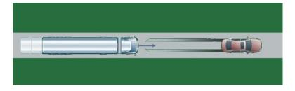
The advanced emergency braking system shall provide the driver with the warning specified in paragraph 2.2.3., and with the driver applying the brakes insufficiently to prevent the collision the braking performance shall be autonomously increased to an appropriate level to prevent the collision.
