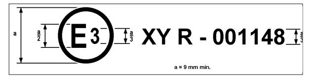
The TBW or TLAS or TPMS bearing the above approval mark is a TBW or TLAS or TPMS that has been approved in Italy (E3) under approval number 001148.
