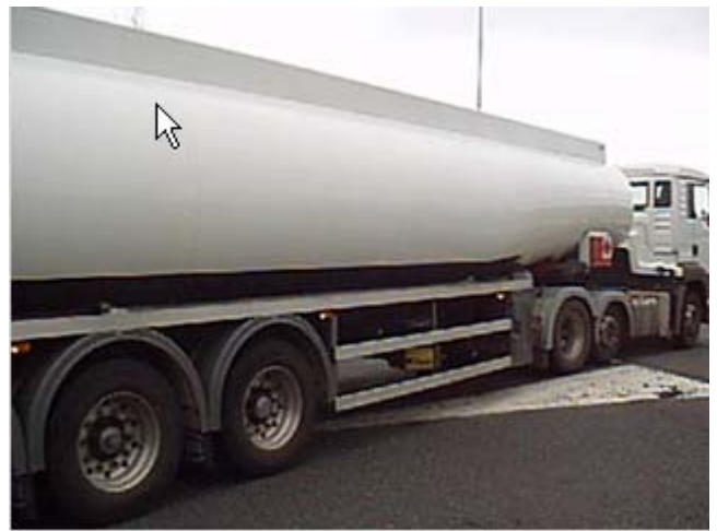
Three side direction indicators fitted to tanker note tanker rear lights obscured by semi-trailer
