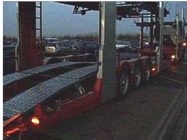
Transporter vehicle fitted with extra side direction indicator to compensate for obscuration of lights when fully laden
