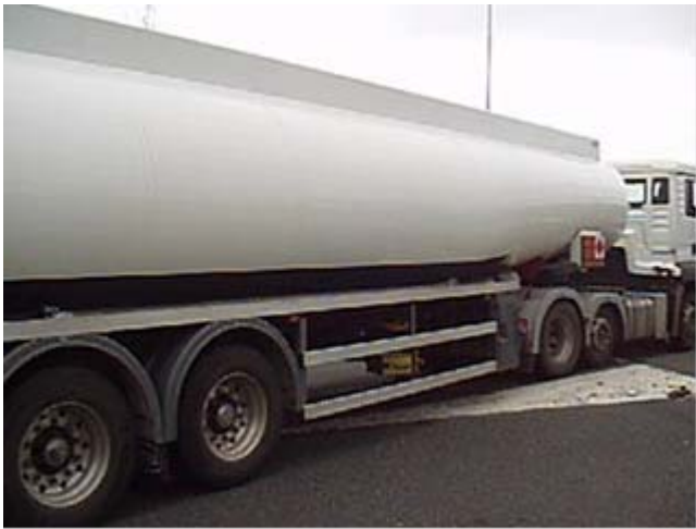
Three side direction indicators fitted to tanker note tanker rear lights obscured by semi-trailer
