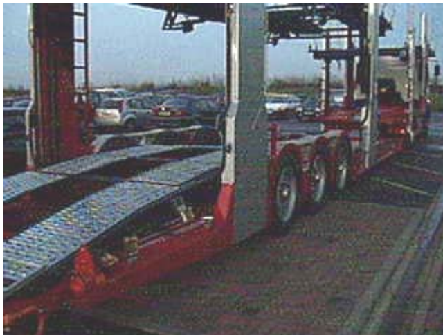
Transporter vehicle fitted with extra side direction indicator to compensate for obscuration of lights when fully laden
