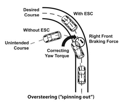
Figure 1: ESC Interventions for Understeering and Oversteering
