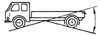
4.7.5.4. "Ground clearance between the axles" means the shortest distance between the ground plane and the lowest fixed point of the vehicle.
